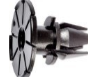
Black Nylon Moulding Clip; 30 Top Head, 18.5 Btm Head, 14 Stem Len, 27 Overall Len
