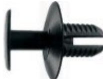
Black Nylon Trim Clip; 15 Head, 20 Flange, 14 Stem Len, Fits 8 Hole
