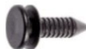
Black Nylon Trim Clip; 12.3 Top Head, 12.3 Btm Head, 5.5 Stem Dia, 17 Stem Len
