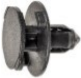
Black Nylon Pin-Type Clip; 16 x 19 Top Head, 20 Btm Head, 12 Stem Len, Fits 8 Hole
