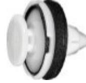
White Nylon Trim Clip w/Top & Btm Sealer; 13 Top Head, 20 Flange, Fits 8 Hole
