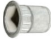
Silver Zinc Coated Tin Insert; 8 Thread Size, .7mm-3.8 Grip, 17 Head, 12.5 Hex
