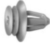
White Nylon Push In Clip; 14 Top Head, 15 Mid Head, 18 Btm Head, 14 Stem Len, 9.5 Stem Dia.
