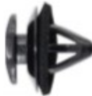
Black Nylon Import Clip; 11 x 14 Top Head, 17 Btm Head, 12 Stem Len, 9.7 Hole
