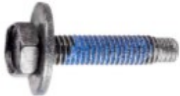
Black Zinc Metric Body Bolt w/Dog Point & Locking Thread; 6 x 30 Thread Size, 10 Hex, 18 Washer
