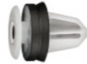
White Nylon Import Clip w/Sealer; 14.5 Top Head, 15 Btm Head, 11 Stem Dia, 15 Stem Len
