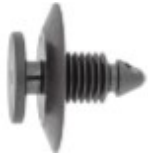
Black Nylon Push-In; 13 Top Head, 21 Btm Head, 7.4 Stem Dia, 14 Stem Len
