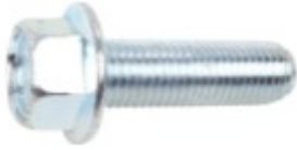
Zinc J.I.S. Hex Flange Head Bolts 8-1.25 x 25, 12 Hex, 17.5 Flange, 10.9 Class
