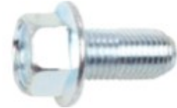
Zinc J.I.S. Hex Flange Head Bolts 10-1.25 x 16, 14 Hex, 20 Flange, 10.9 Class
