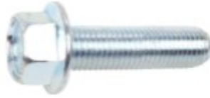
Zinc J.I.S. Hex Flange Head Bolts 8-1.25 x 30, 12 Hex, 17.5 Flange, 10.9 Class
