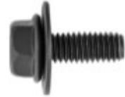
Black Phosphate Metric Body Bolt 6-1.0 x 15 Thread, 10 Hex, 18 Washer
