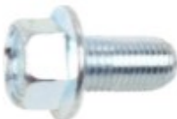
Zinc J.I.S. Hex Flange Head Bolts 8-1.25 x 12, 12 Hex, 17.5 Flange, 10.9 Class
