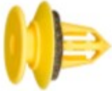
Yellow Nylon Push-In Clip w/Sealer 15 Top Head, 17 Btm Head, 9 Stem Dia, 14 Stem
