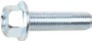
Zinc J.I.S. Hex Flange Head Bolts 10-1.25 x 35, 14 Hex, 20 Flange, 10.9 Class
