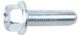
Zinc J.I.S. Hex Flange Head Bolts 10-1.25 x 30, 14 Hex, 20 Flange, 10.9 Class
