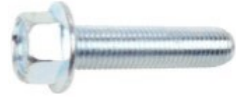
Zinc J.I.S. Hex Flange Head Bolts 8-1.25 x 35, 12 Hex, 17.5 Flange, 10.9 Class
