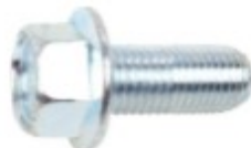
Zinc J.I.S. Hex Flange Head Bolts 8-1.25 x 16, 12 Hex, 17.5 Flange, 10.9 Class
