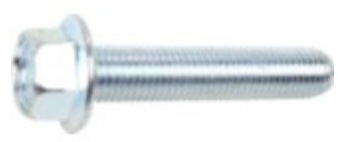
Zinc J.I.S. Hex Flange Head Bolts 10-1.25 x 45, 14 Hex, 20 Flange, 10.9 Class
