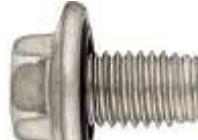
Zinc Oil Drain Plug with Rubber Gasket M12-1.75 Thread, 15 Hex w/ T45 IntD, 17 LUHD,
