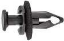
Black Nylon Push-Type Clip With Sealer 15 HD, 21 StL, Fits 8 Hole
