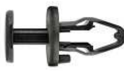
Black Nylon Push-Type Clip With Sealer 14 HD, 18 StL, Fits 8 x11 Hole
